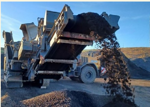
Mobile aggregate crushing and screening unit processing waste that was generated from Cornwall's highway network.
