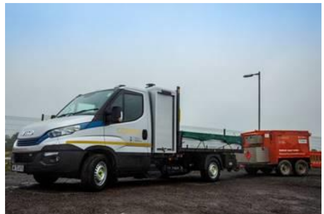
Cormac's new bio-methane powered highway maintenance vehicle and pot-hole repair trailer.
